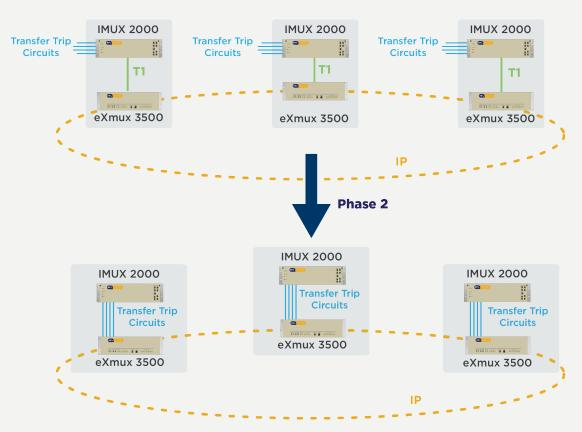
Figure 2: Plase 2 in a staged upgrade from a linear to a redundant ring network
