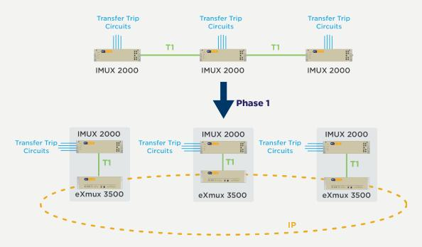
Figure 1: Phase 1 in a staged upgrade from a linear to a redundant ring network
